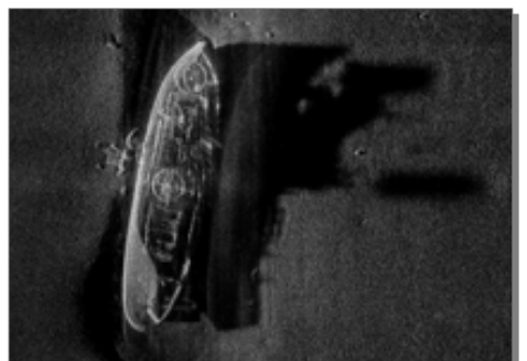
Top: The CRV Leonardo (left) and the NRV Alliance (right). Middle: Two autonomous underwater vehicles being launched from the Alliance. Bottom: Synthetic Aperture Sonar (SAS) was used to produce this detailed image of a sunken ship.
